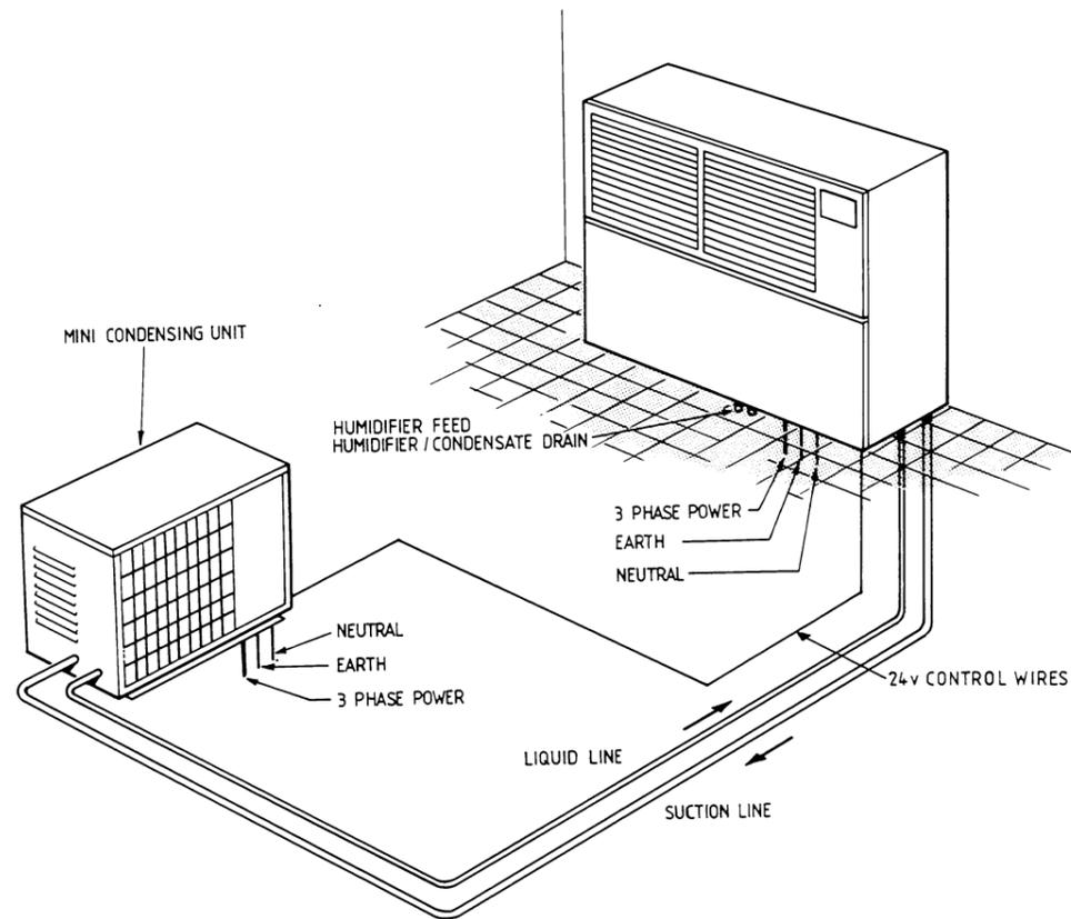
Schematic Interconnection Diagram - EMDFA/EMVA
