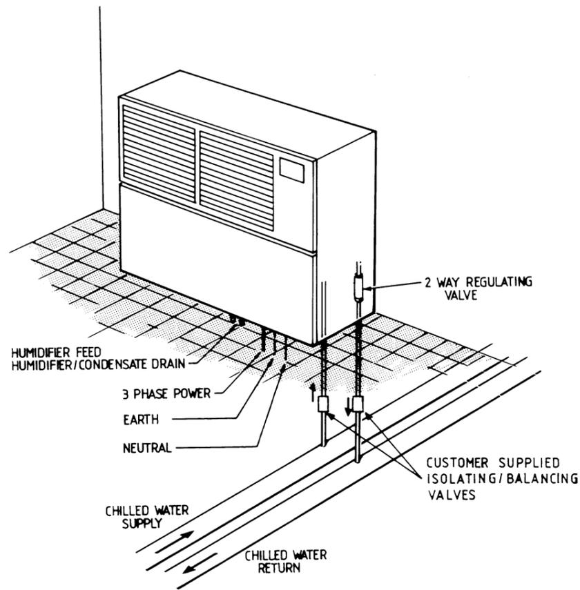
Schematic Interconnection Diagram - Chilled Water
