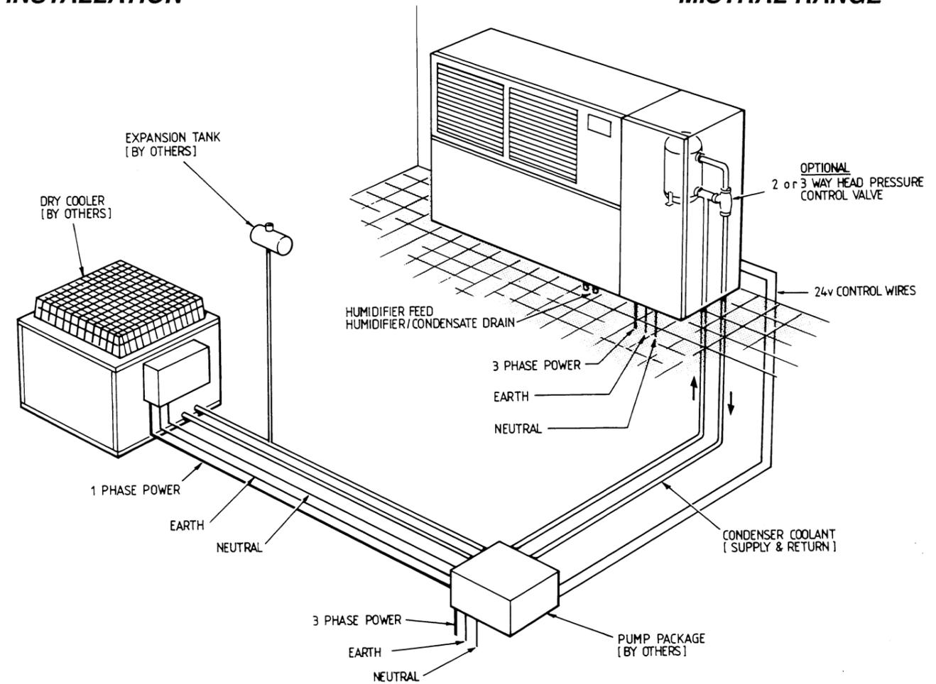
Schematic Interconnection Diagram - EMDFW/EMVW
